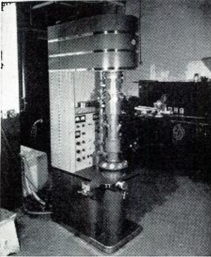
Latest electron discovery, the electronic microscope. Uses cathode rays.
